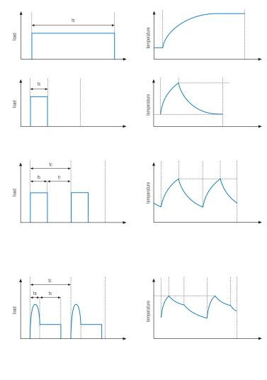
A motor designed for S1 duty but running on S2 or S3 duty can provide a power output higher than the rated one on S1 duty. However, the starting torque remains the same on all duties. The permissible approximate output power for single speed motors can be calculated as follows:
